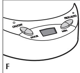
1. To set current time of day: Press the HOUR button, little dot in the top left corner of the display indicates the "p.m." time. Press the MIN button. Once set, clock continues to keep time unless coffeemaker is unplugged or a power failure occurs. Clock can only be reset when in the flashing mode (F).
