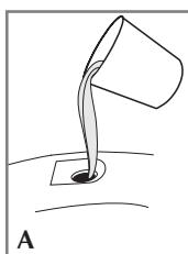
1. Tilt the iron and using a clean measuring cup, pour water into opening until the water reaches the MAX level mark on the water tank (A). Do not overfill. Refill as needed.
