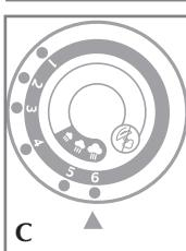
2. Turn the fabric-select dial to appropriate setting (between 4 and 6) for your fabric (C). See fabric guide on the heel rest and read garment's label to help you determine fabric type. The temperature-ready light glows until it reaches the appropriate temperature. It then cycles on and off during ironing.
