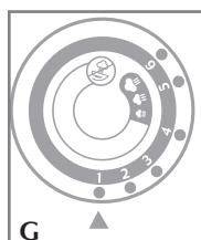
2. Turn the fabric-select dial to the appropriate setting for your fabric (**G**). See fabric guide on the heel rest and read garment's label to help you determine fabric type. The temperature-ready light glows until it reaches the appropriate temperature. It then cycles on and off during ironing.
