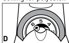
2. Once you determine the fabric type, turn the fabric select dial at the front of the handle clockwise to select the appropriate fabric setting (D).
