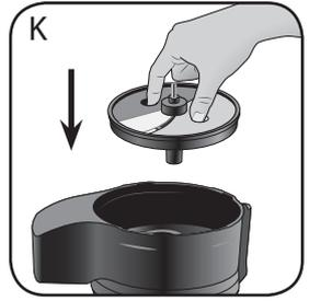
**Note:** Position slicing disc blade just to the right of the feed chute. This allows the blade a full rotation before contacting the food.
