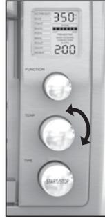
2. Using the TEMP knob, adjust temperature.
