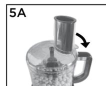
**If using chopping blade:** put food into work bowl below the max food level. Place cover on work bowl as shown and rotate clockwise. Put the food pusher in place.
