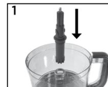
With unit unplugged from outlet, place workbowl on base and put the center shaft in workbowl.
