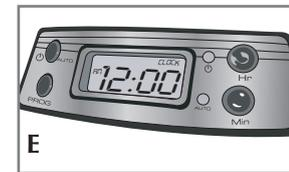
3. Press the Program button; the word Clock appears on the top right of the display (E).
