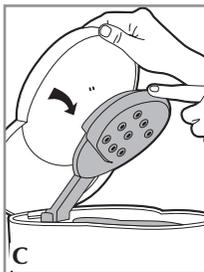
2. To clean inside the reservoir cover, pull the water spreader down (C), wipe the surfaces with a damp cloth, and snap the water spreader back into place.
