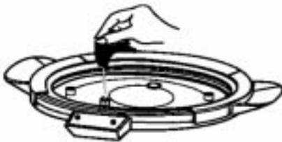
Clean the Sensor Pad (located on bottom of Removable Cooking Pot) after each use.
