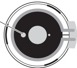
8. In order to maintain the good performance of your Pressure Cooker, the bottom of the Removable Cooking Pot, in the area of the Sensor Pad, must be cleaned after each use. The Sensor must be free of dirt, food, or residue. To do so, wipe with a soft, damp cloth and be sure to dry thoroughly.
