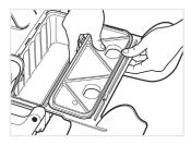
5. Attach the waste receptacle lid by inserting the pushtabs into the round holes. To secure, press on the positions indicated.
